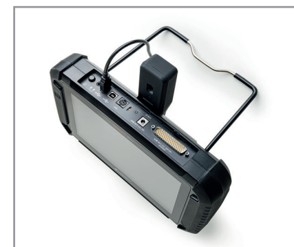
The Smart Programmer connects to the rear of the Smart Pro via the USB cable
