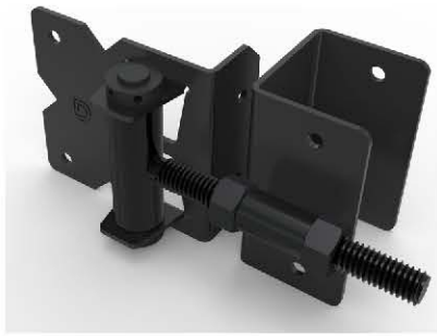
DDS2HNW3A/DDS2HNW3AW Regular Hinge. Self-closing, tension adjustable. Standard to 51mm (2") wrap-around
