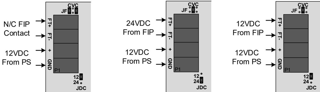
If a normally closed fire trip is used care must be taken to set JDC to the value of the power supply input as this will be used to activate the fire relay.
