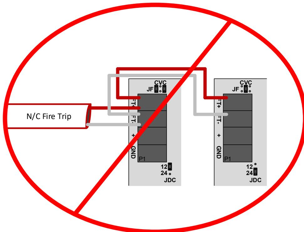
**Note:** A normally closed contact cannot be used in parallel to drive multiple fire trip relays directly. Instead, downstream fire trips should use either the expansion voltage or a dry contact from the AA terminals of an upstream Power Port module. Take care to correctly set JF and JDC.
