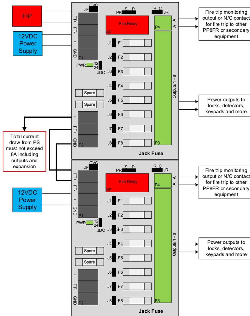
**Additional outputs.** Additional fused power outputs can be added using the expansion boards PP10HD or PP10MG. One or more boards can be added if the total current drawn via the PP8PTC does not exceed the PCB or fire relay limit of 8A. If current draw exceeds limitations an additional PP8FR module can be used.
