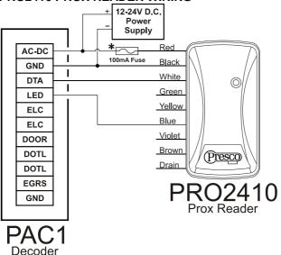
**Note** that the Green, Yellow, Violet, Brown and Drain wires are not connected when the PRO2410 is used with a PAC1 decoder.
