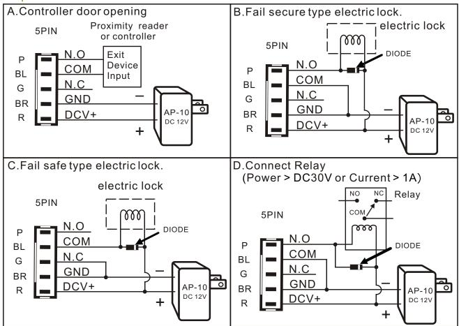
\*Please connect to diode when the control terminal is loading in order to absorb surge to prevent damage to the sensor.
