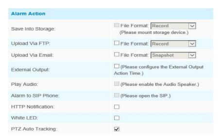
Step6: Set alarm settings. If you enable External Output and choose Constant External Output Action Time, when detected object is marked as "person", External Output Action alarm time will
