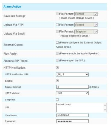
Step7: Set alarm settings. If you enable External Output and choose Constant External Output Action Time, when the thresholds exceeds the certain value you set, External Output Action alarm time will be always constant till the alarm is released.
