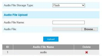
Note:Only support '.wav' audio files with codec type PCM/PCMU/PCMA, 64kbps or 128kbps bitrate and no more than 500k!
