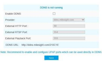
You can choose "ddns.milesight.com" as provider for DDNS. After enabling, you can access the device via the URL "http://ddns.milesight.com/MAC address".
