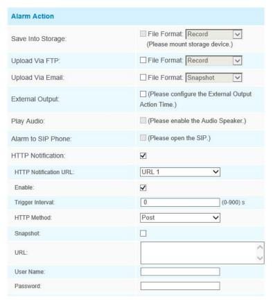
Step4: Set alarm settings. If you enable External Output and choose Constant External Output Action Time, when possible tampering is detected, External Output Action alarm time will be always constant till the alarm is released.
