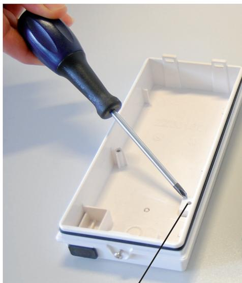
**Screw for Anti-removal system - Fig.1**
